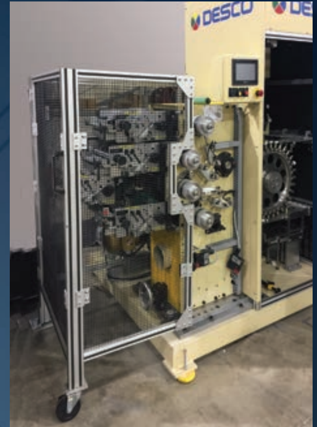
Steel Cage Print Tower Machine Mount Enclosure with Interlock Doors Front and Back
